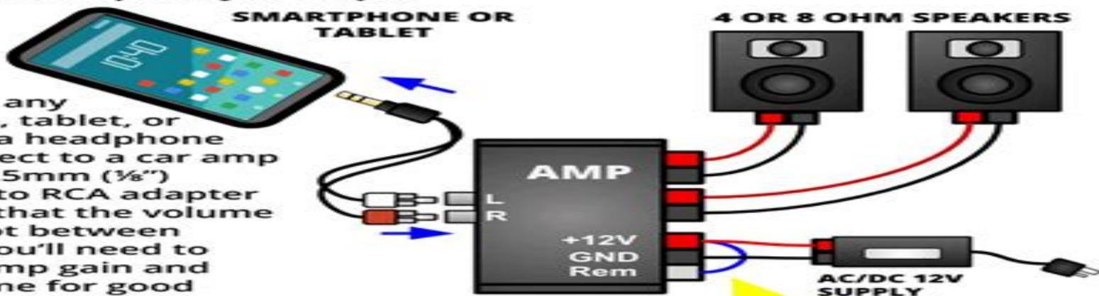
You can use any smartphone, tablet, or laptop with a headphone jack to connect to a car amp by using a 3.5mm ( $\frac{1}{8}$ " ) headphone to RCA adapter cable. Note that the volume can vary a lot between devices so you'll need to adjust the amp gain and device volume for good sound.
