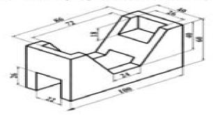
Draw a complete orthographic drawing of the right solids shown in figure cut by the planes. Find the true shape of the section and draw total surface development of the solid.
