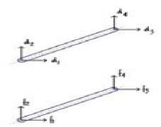
For finite element of the bar:
