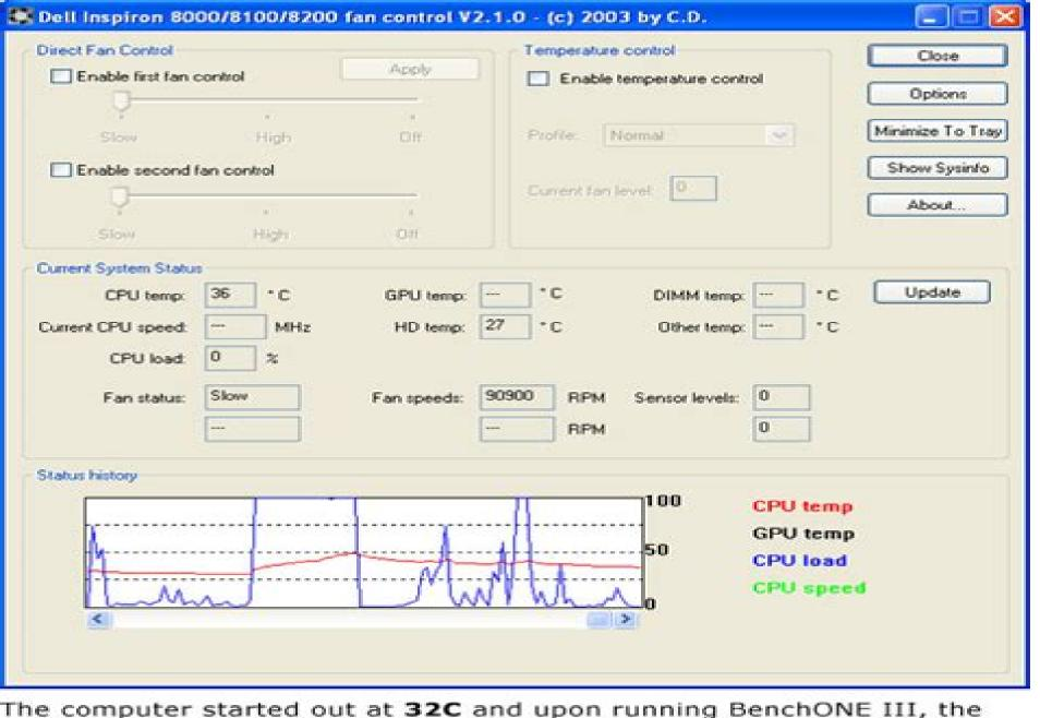
cpu usage went to 100% for about 1 minute, at which time, the temp. peaked at **48C**. Afterwaards, it cooled down to **36C** as shown above. btw, my BenchONE score went from 8933 to 9909...1000 point increase!
