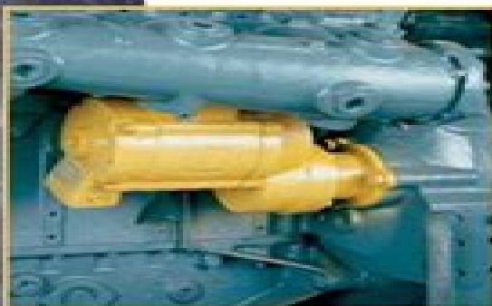
IR's genuine SS810GB03R31R inertia remanufactured starter is shown mounted on a Detroit Diesel 16V-71R.
