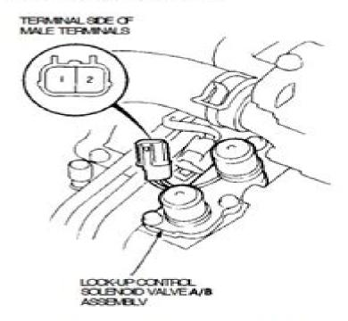
Measure the resistance between the No. 2 terminal solenoid valve A) of the lock-up control solenoid valve connector and body ground, and between the No. 1 terminal (solenoid valve B) and body ground.
