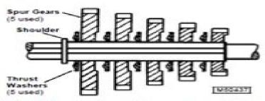
Install thrust washers and spur gears on shaft from brake splines end with raised side of thrust washers toward shoulder of shaft. Flat side of gears MUST BE toward shoulder.
