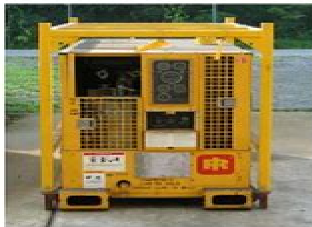
175-Cfm Air Compressor Controls and Gauges
