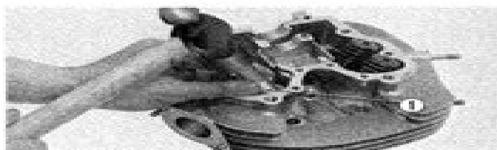
Fig. 1-9 ① Valve guide driver (07942-3290200)
