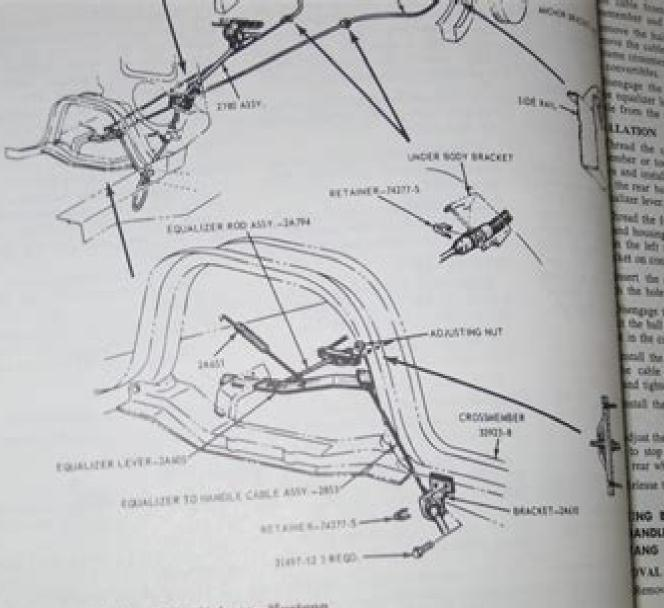
FIG. 27-Perking Brake Linkegs-Hustong
