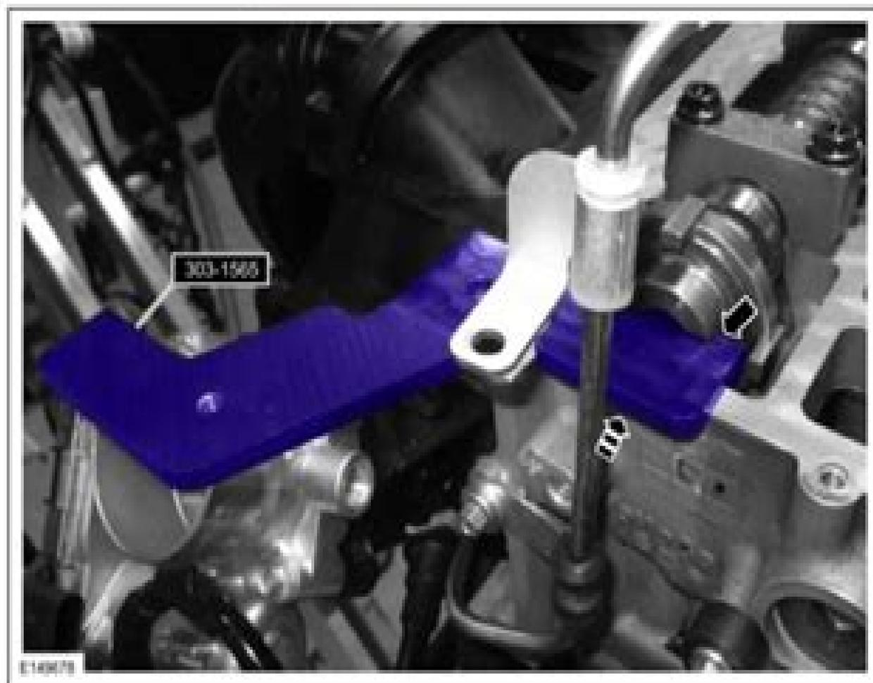
10. **NOTE:** The crankshaft must remain in the TOP position during removal of the pulley bolt or damage to the engine can occur. Therefore, the crankshaft pulley must be held in place with the special tool, and the crankshaft pulley bolt should be removed using an air impact wrench (1/2-in drive minimum).
