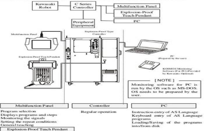
Program selection Programs and steps Display Manual operation of the robot Monitoring the signals Setting the repeat conditions Positional teaching General teaching
