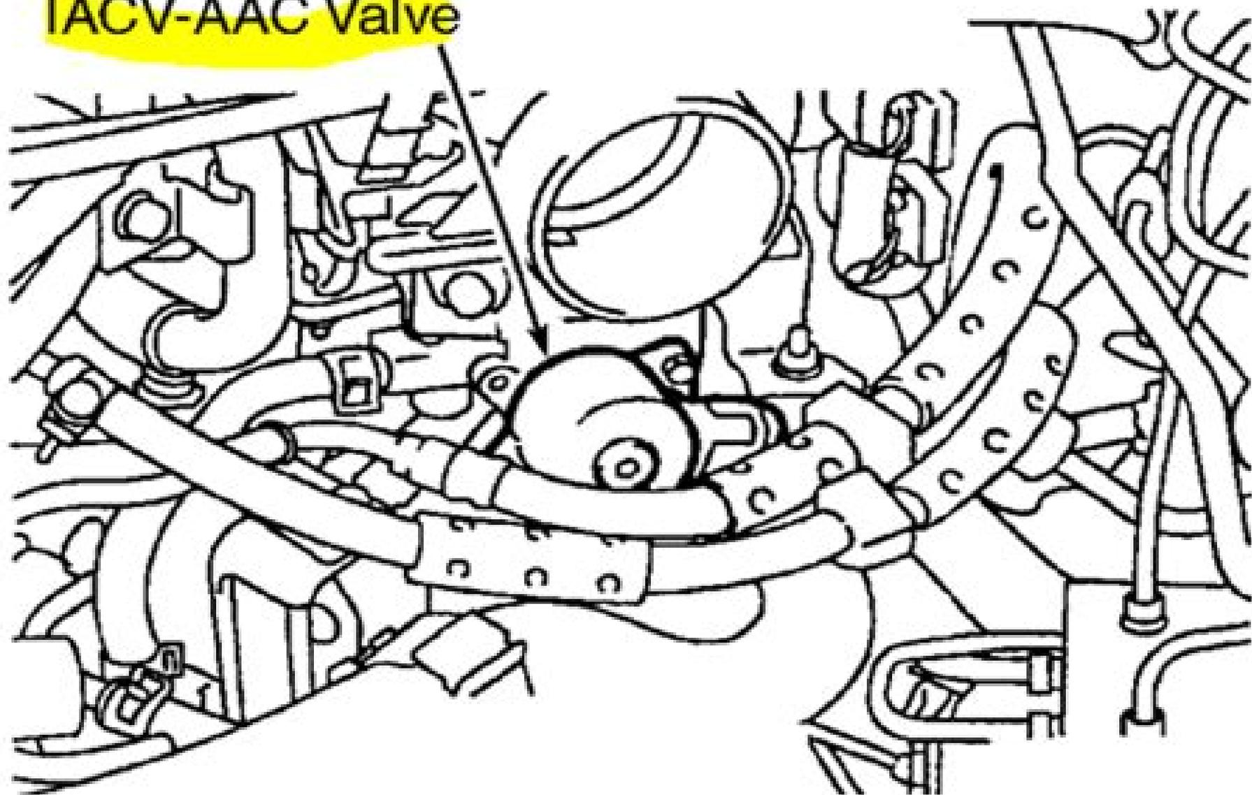
VIEW WITH INTAKE AIR DUCT REMOVED
