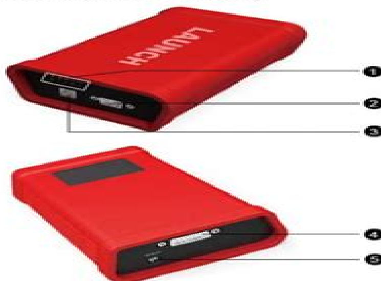
Fig. 5-1 Ports and indicators of X-431 HD module
