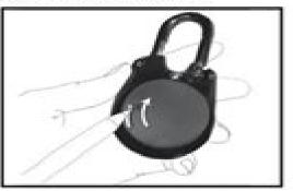
On the back of the lock, use a pointed object to slide the reset lever into the "up" position (toward the "R").
