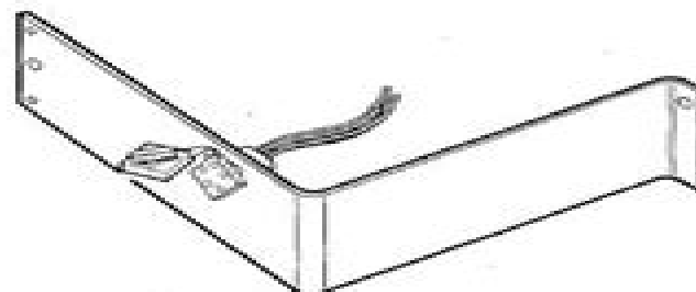
Fig. 2. Proper Installation of Female Receptacle Plug
