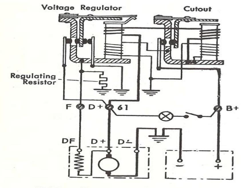
Wiring diagram of the regulator.
