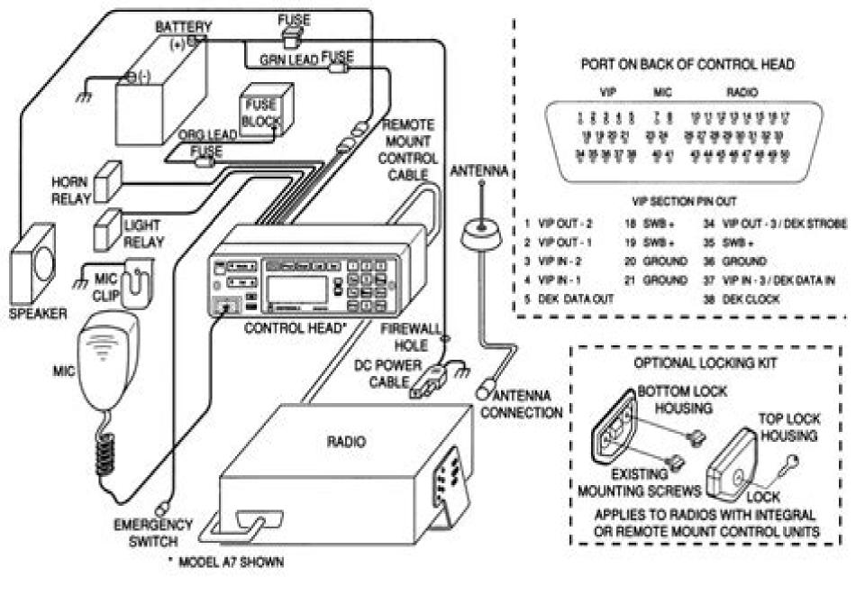
Figure 4. Low-/Mid-Power Radio Installation (Remote) Using A4, A5, A7 or A9 Control Heads
