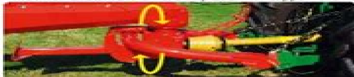
The Gyrodine swivel hitch: 540 or 1000 min -1
