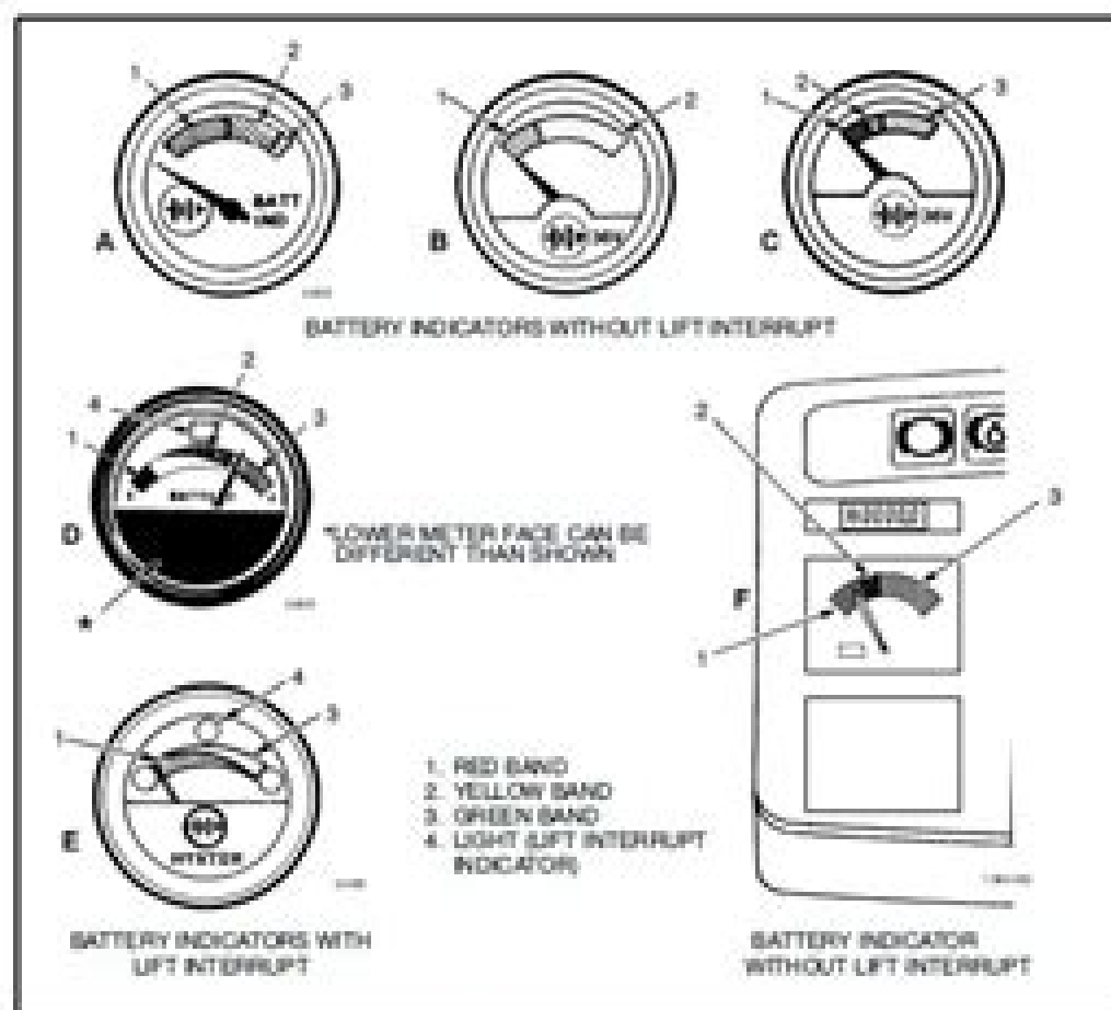
FIGURE 1. BATTERY INDICATORS WITH METER MOVEMENTS
