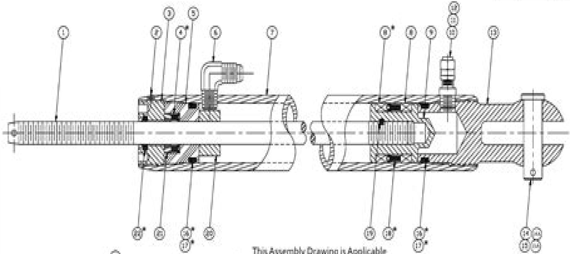
This Assembly Drawing is Applicable to all SE, LE and FE HP Cylinders.
