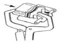
NOTE: Brake fluid will be forced through compensating port into master cylinder fluid reservoir when piston is pushed back into caliper. Remove excess fluid from reservoir as required.
