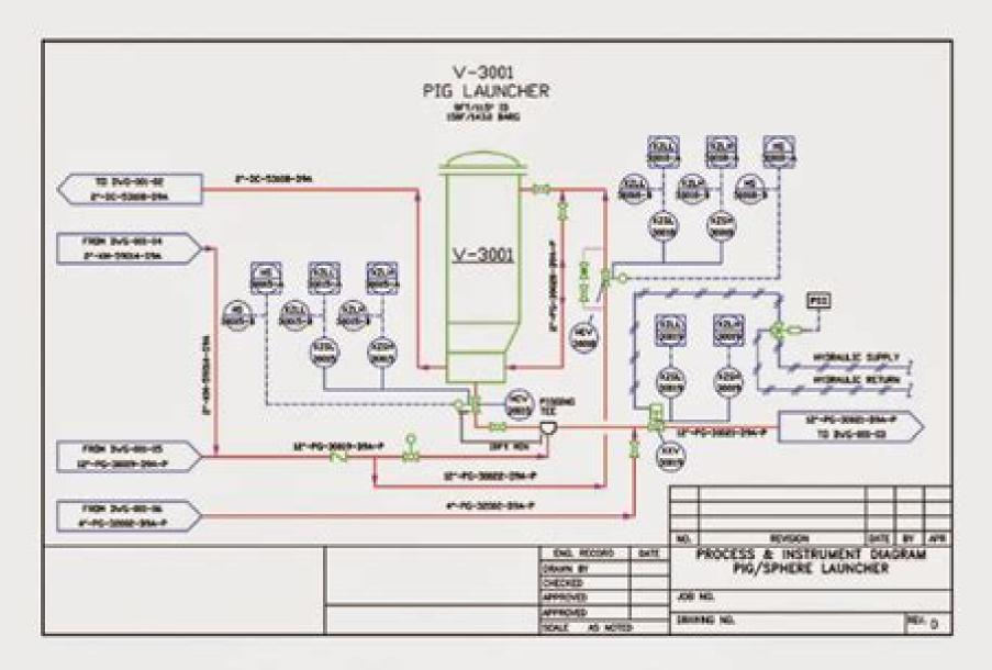
Piping and instrumentation diagram
