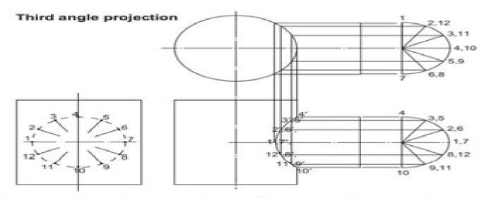
2. A vertical cylinder of diameter 60 mm is fully penetrated by a cylinder of diameter 45 mm, their axes intersecting each other. The axis of the penetrating cylinder is inclined at 30 to the HP and is parallel to the VP. Draw the top and front views of the cylinders and the curves of intersection.
