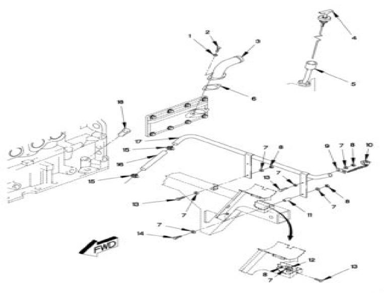
FIGURE 21. ENGINE OIL DIPSTICK AND FILLER TUBE
