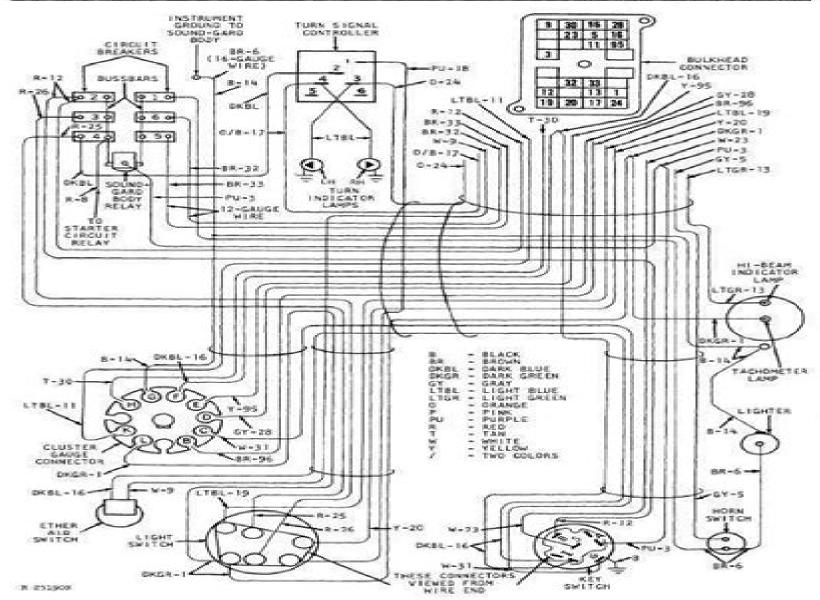
Fig. 18-Main Instrument Harness Connections
