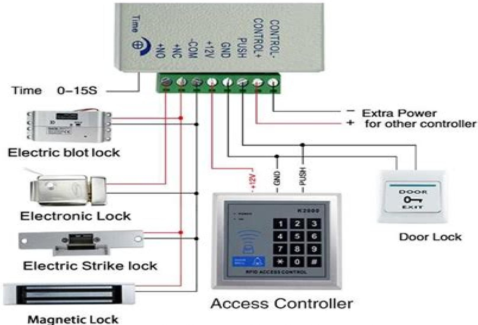
Attention when electronically controlled lock must be transferred to 0 seconds delay, to prevent burning of electric lock.
