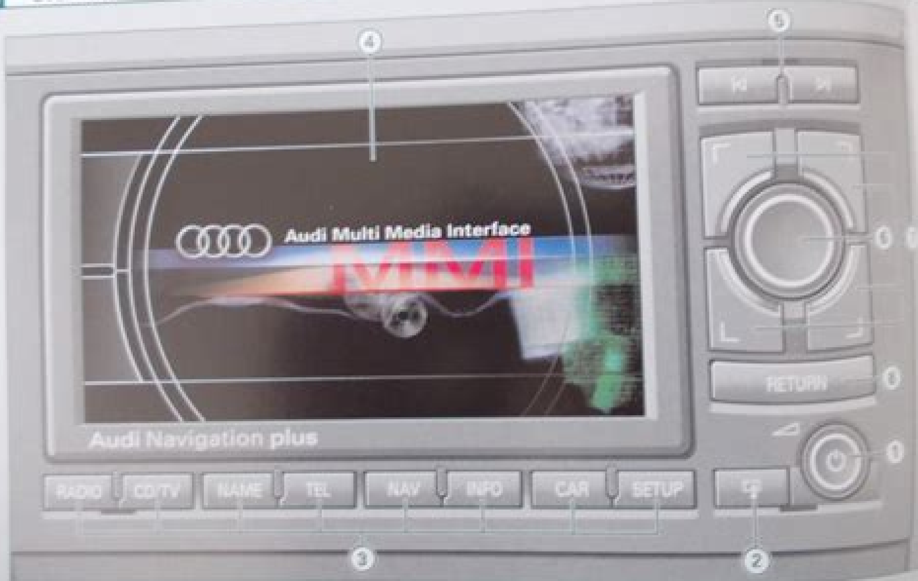
Fig. 1 Control console: Audi Navigation plus
