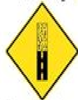
Paved surface ends
