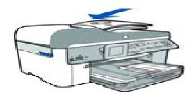
Slide paper-width guide inward until it stops at edge of paper.
