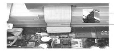
Snap the Locking Clips over the top of the connector to secure the Ribbon Cable
