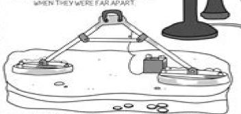
HE ALSO INVENTED A DEVICE CALLED THE METAL DETECTOR IT WAS ORIGINALLY CREATED TO HELP FIND A BULLET IN PRESIDENT GARFIELD'S BODY AFTER HE WAS SHOT. THE METAL DETECTOR COULD LOCATE METAL OBJECTS HIDDEN INDER THE GROUND, TODAY, METAL DETECTORS ARE USED IN VARIOUS WAYS, SUCH AS FINDING LOST TREASURES LOCATING PIPES AND WIRES UNDERGROUND, AND EVEN FOR SECURITY PURPOSES AT AIRPORTS
