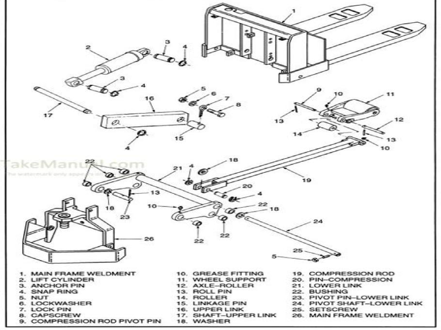
FIGURE 2 - EXPLODED VIEW LIFTING MECHANISM
