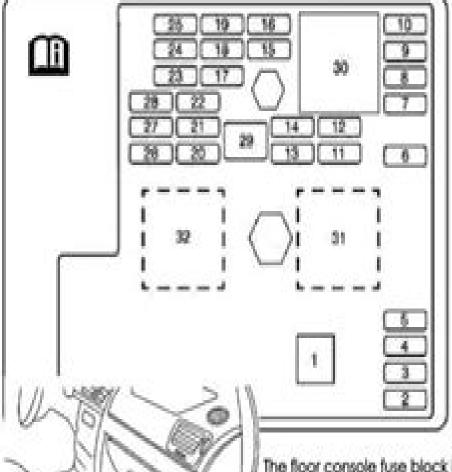
The floor console fuse block is located on the passenger side of the floor console behind the forward panel. The panel has four clips, one in each corner. Pull the panel to disconnect the four clips, and access the fuses.
