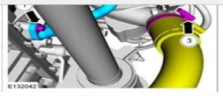
Black arrows are used to draw attention to components (usually fasteners). Arrows with multiples specified (here, x2) identify an identical number of fasteners or items. Callouts (numbers inside circles) show a required sequence or tightening torque.
