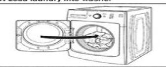
Place a load of sorted clothes loosely in the washer, items need to move freely for best cleaning and to reduce wrinkling and tangling. Close the washer door by pushing it firmly until the latch clicks.
