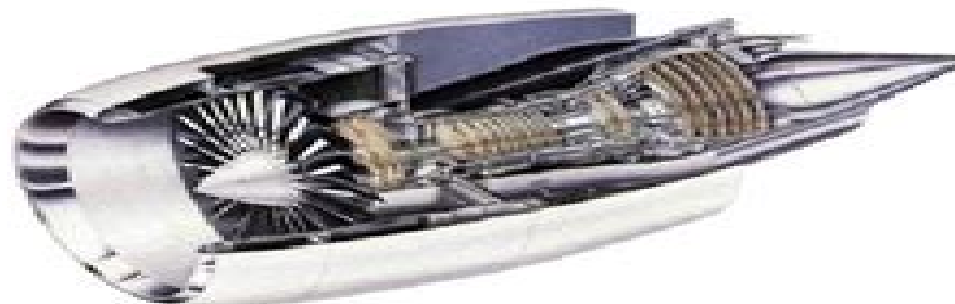
GE-90 TURBOFAN ENGINE (CUT-AWAY VIEW)
