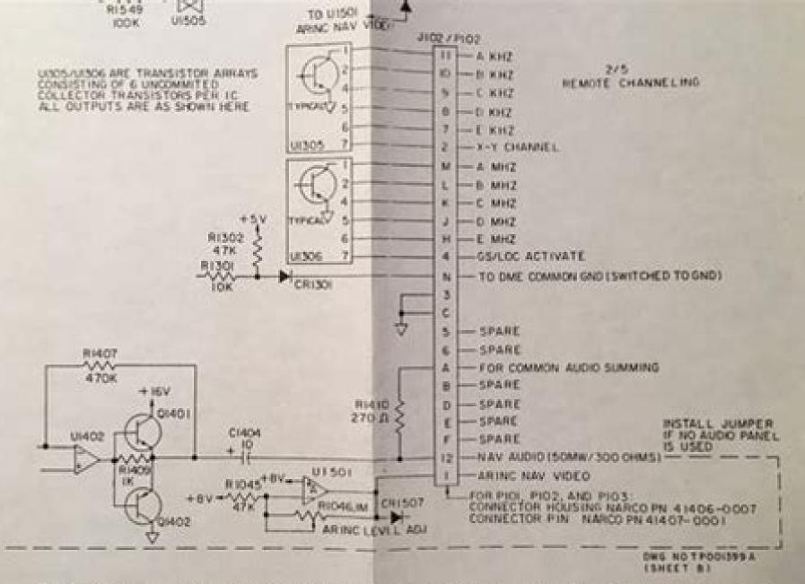
FIGURE 2-3. MK-12D EXTERNAL INTERCONNECT DIAGRAM P101, P102, P103
