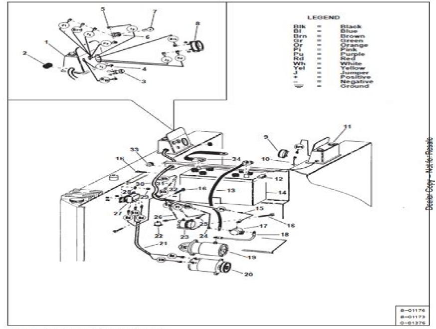
Fig. 62 Main Frame Electrical Circuit (444 Gasoline)
