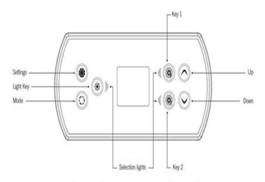
\*Functions for keys 1 and 2 will depend on your system's low level configuration.
