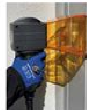
Remove screws of focusing hood
