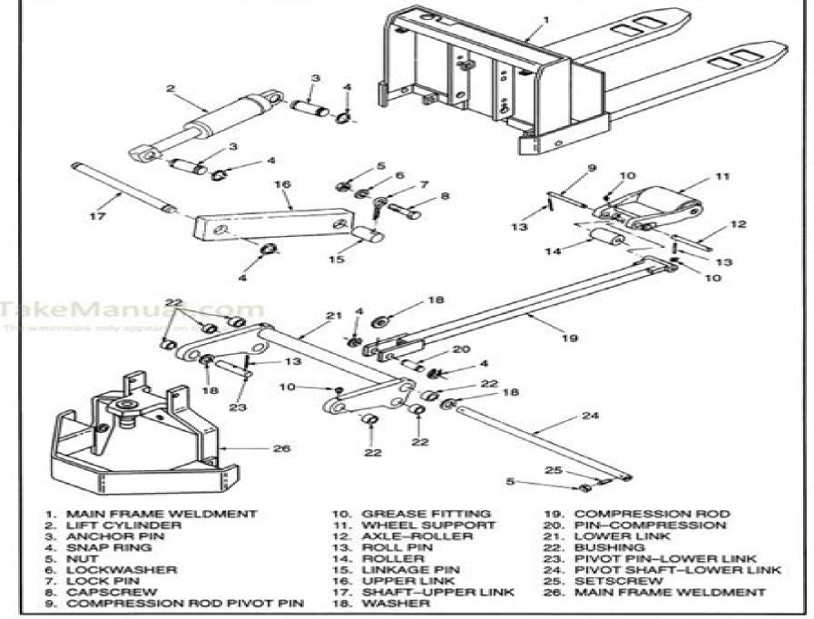
FIGURE 2 - EXPLODED VIEW LIFTING MECHANISM
