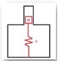
Helmholtz resonator is a side branch acoustic absorber.
