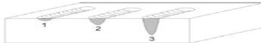
Figure F. Three types of welds created according to the power density and pulse duration of the laser pulse.
