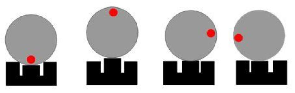
DISPLACEMENT OF THE BULLET WHEN THERE IS ANGULAR SHIFT ERROR IN THE ALIGNMENT OF THE FRONT SIGHT.
