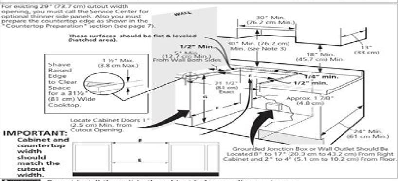
TYPE Do not install the unit in the cabinet before reading next page.
