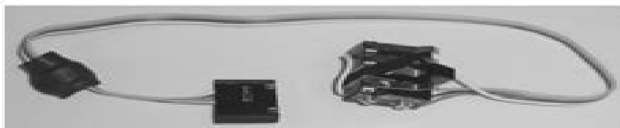
Figure 1 – Shunt Switch Assembly (P/N M42408)
