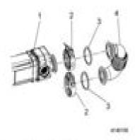
3. Remove the mixer pipe (4) from the cold baset pipe (1). Role to section.
