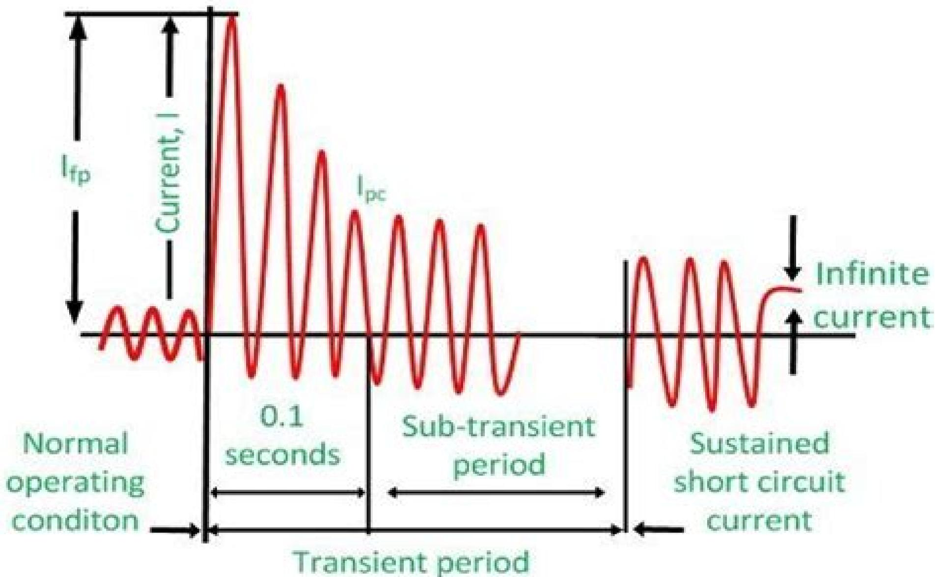
Process of Change in a Short-Circuit Current
