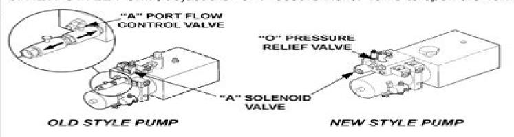
2. Check the "A" Solenoid Valve Coil for power. Place a screwdriver about 1/4" from the "A" Solenoid and energize the unit. If the screwdriver is not drawn to the energized solenoid the solenoid must be repaired or replaced.
